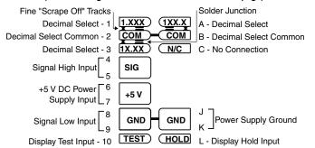
**Pins A, 1 and 3 - Decimal Select:** Decimal points may be blanked as required by carefully scraping off the fine tracks linking these pins to Decimal Select Common using a pair of pliers or a small screwdriver blade. Re-connect either by linking the appropriate pins on the connector or by solder-bridging the junctions located on the PC board edge fingers.
